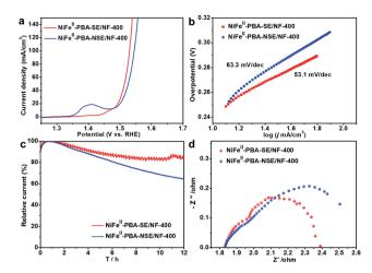
Fig. 5 (a) IR-corrected linear sweep voltammetry (LSV) curves, (b) corresponding Tafel plots of the catalysts with and without encapsulation, and (c) the durability measurements of NiFe<sup>II</sup>-PBA-SE/NF-400 and NiFe<sup>II</sup>-PBA-NSE/NF-400 under a constant potential of 1.6 V (vs. RHE). (d) Nyquist plots of the catalysts with and without encapsulation with a potential of 1.6 V (vs. RHE).
