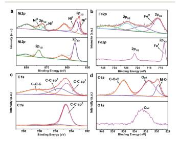
Fig. 3 XPS spectra of (a) Ni 2p, (b) Fe 2p, (c) C 1s and (d) O 1s for initial NiFe $^{II}$ -PBA and NiFe $^{II}$ -PBA-SE/NF-400 (with the bottom spectra corresponding to initial NiFe $^{II}$ -PBA without heat treatment and the upper spectra corresponding to NiFe $^{II}$ -PBA-SE/NF-400).
