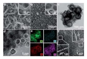
Fig. 2 SEM images of (a) initial NiFe<sup>II</sup>-PBA/NF without heat treatment, (b) NiFe<sup>II</sup>-PBA-SE/NF-400, (c, d, f) HRTEM images and (e) the elemental distribution mapping of NiFe<sup>II</sup>-PBA-SE/NF-400.
