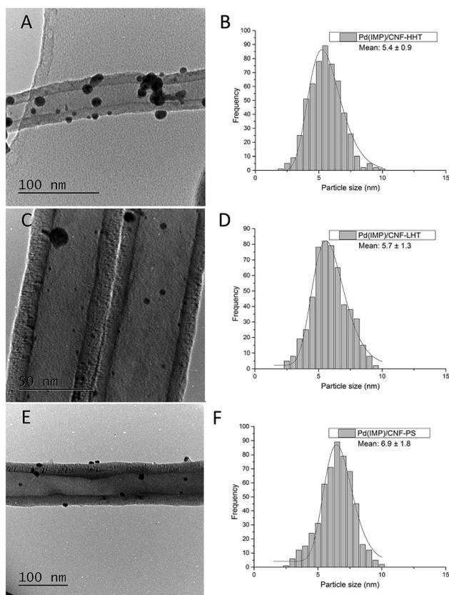
Fig. 6 Bright field TEM micrographs and corresponding histograms of the particle size distributions for the fresh catalysts prepared by impregnation. (A and B) Pd<sub>IMP</sub>/CNF-HHT, (C and D) Pd<sub>IMP</sub>/CNF-LHT, and (E and F) Pd<sub>IMP</sub>/CNF-PS.
