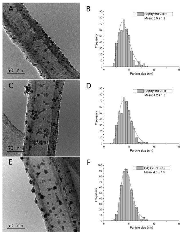
Fig. 7 Bright field TEM micrographs and corresponding histograms of the particle size distributions for the fresh catalysts prepared by sol-immobilisation. (A and B) Pd<sub>SI</sub>/CNF-HHT, (C and D) Pd<sub>SI</sub>/CNF-LHT, and (E and F) Pd<sub>SI</sub>/CNF-PS.
