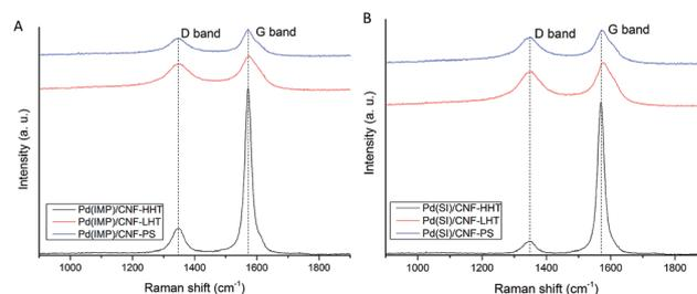
Fig. 5 Raman spectra of the fresh samples. (A) Catalysts synthesised by impregnation: Pd<sub>IMP</sub>/CNF-HHT (black curve), Pd<sub>IMP</sub>/CNF-LHT (red curve) and Pd<sub>IMP</sub>/CNF-PS (blue curve). (B) Catalysts synthesised by sol-immobilisation: Pd<sub>SI</sub>/CNF-HHT (black curve), Pd<sub>SI</sub>/CNF-LHT (red curve) and Pd<sub>SI</sub>/CNF-PS (blue curve).
