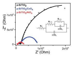
Fig. 5 Nyquist plots of p-Si/TiO<sub>2</sub> (black), p-Si/TiO<sub>2</sub>/CoO<sub>x</sub> (blue), p-Si/  $TiO_2/NiO_x$  (red) measured at 0.0  $V_{RHE}$  under 1 sun illumination. The inset shows the equivalent circuit employed for analyzing the Nyquist plots. The fit data are provided in ESI Table S2.†
