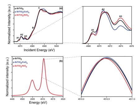
Fig. 7 X-ray spectroscopy characterization of p-Si/TiO<sub>2</sub> (black), p-Si/TiO<sub>2</sub>/CoO<sub> $_X$ </sub> (blue), p-Si/TiO<sub>2</sub>/NiO<sub> $_X$ </sub> (red): (a) HERFD-XANES spectra acquired at the Ti K-edge. The magnified view on the right shows the pre-edge peaks. (b) Kα emission lines. The magnified view on the right shows the Kα peak maximum.
