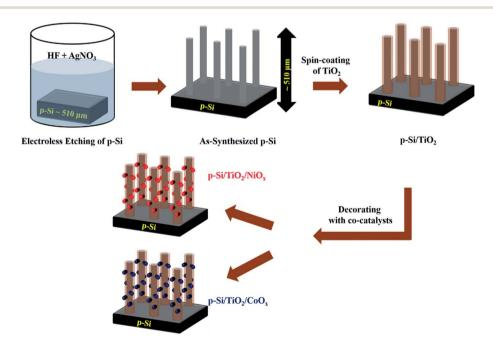
Fig. 1 Schematic representation (not to scale) of the preparation steps of p-Si micro-wires by wet-etching, their coating with  $TiO_2$  and subsequent functionalization with  $NiO_x$  or  $CoO_x$  via spin coating and sintering. The procedure is described in detail in the ESI.†
