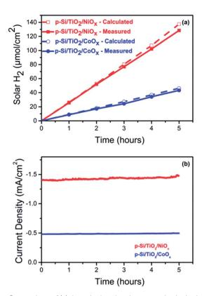
Fig. 4 Comparison of (a) the calculated and measured solar hydrogen production per geometric surface area of the photoelectrode and (b) of the current density of  $\mathrm{NiO}_x$  (red) and  $\mathrm{CoO}_x$  (blue) functionalized p-Si photo-electrodes over 5 hours of continuous operation. The data displayed in (a) and (b) were obtained simultaneously at 0.0  $\mathrm{V}_{\mathrm{RHE}}$  and 1 sun illumination.
