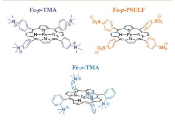
Fig. 2 Iron tetraphenylporphyrin derivatives with positive and negative charges used for electrocatalytic reduction of  $\rm CO_2$  to  $\rm CO$ . Reprinted with permission from ref. 88. Copyright 2016, American Chemical Society.
