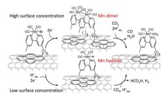
Scheme 10 Two-electron reduction of  $CO_2$  to CO vs. HCOOH with the [MnBr(2,2'-bipyridine)(CO)<sub>3</sub>] complex anchored to a carbon nanotube electrode via a pyrene unit depending on the surface concentration. Reprinted with permission from ref. 134. Copyright 2017, American Chemical Society.
