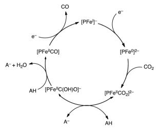
Scheme 3 Catalytic cycle for two-electron reduction of  $CO_2$  to CO with an iron porphyrin ([PFe $^1$ ] $^-$ ).<sup>84</sup>
