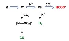
Scheme 7 The reaction pathway of two-electron reduction of  $\rm CO_2$  with a metal complex (M) to produce  $\rm HCOO^-$  or CO. Reprinted with permission from ref. 125. Copyright 2017, American Chemical Society.
