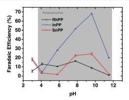
Fig. 9 Faradaic efficiencies for the electrocatalytic reduction of  $CO_2$  to HCOOH or HCOO $^-$  with RhPP, InPP and SnPP, determined at  $t=10\,$  min, at  $E=-1.5\,$  V vs. RHE as function of pH. Reprinted with permission from ref. 126. Copyright 2017, Elsevier.
