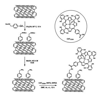
Scheme 4 An iron tetraphenylporphyrin bearing six pendant OH groups in *ortho* and *ortho'* positions on three of the phenyl rings and one carboxylic acid group in the *para* position of the fourth phenyl covalently attached to MWCNTs. Reprinted with permission from ref. 94. Copyright 2016, Royal Society of Chemistry.
