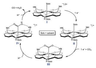
Scheme 5 Catalytic cycle of two-electron reduction of  $CO_2$  to CO with a nonheme cobalt complex with a macrocyclic aminopyridine (I). Reprinted with permission from ref. 96. Copyright 2016, American Chemical Society.
