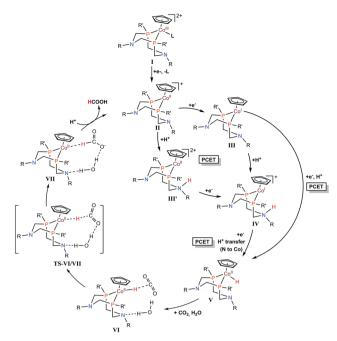
Scheme 9 Catalytic cycle for two-electron reduction of  $CO_2$  to CO with  $[CpCo(P_2^RN_2^R)]I^+$  complexes containing diphosphine ligands  $(P_2^RN_2^R)$  with two pendant amine residues. Reprinted with permission from ref. 133. Copyright 2017, American Chemical Society.
