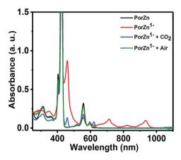
Fig. 5 Absorption spectra of ZnTPP (black line), its reduced species (red line) produced by the reduction of ZnTPP by sodium naphthalenide, and the reduced species after exposure to  $CO_2$  (blue line) or air (green line) in THF. Reprinted with permission from ref. 95. Copyright 2017, American Chemical Society.
