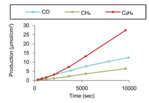
Fig. 12 Products derived from  $CO_2$  electrochemical reduction by crystalline CuPc/C at -1.6 V vs. Ag/AgCl in a two-compartment H-cell. Reprinted with permission from ref. 148. Copyright 2017, American Chemical Society.
