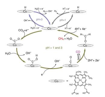
Scheme 12 Catalytic cycle for two electron reduction of  $CO_2$  to CO and further reduction to  $CH_4$  with a Co protoporphyrin molecular catalyst (CoPP) immobilized onto a pyrolytic graphite (PG) electrode (CoPP-PG). Reprinted with permission from ref. 147. Copyright 2015, Nature Publishing Group.
