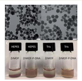
**Fig. 1** (a) Synthesized ZrMOF nanoparticles in DMF. (b) Aptamer conjugated ZrMOF nanoparticles (ZrMOF–P-aptamer) in water. (c) Stability test of ZrMOF nanoparticles and aptamer-conjugated ZrMOF nanoparticles in HEPES and Tris buffers. Scale bar: 100 nm.
