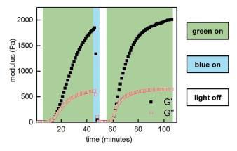
Fig. 6 Photocontrolled cycling of hydrogel viscoelasticity (10% strain, 25 rad s $^{-1}$ ) of P1 and P2-F<sub>2</sub> (1:1, 10 w/v% in PBS, pH 7.5). Green light induces gelation, and blue light induces softening.
