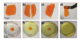
Fig. 7 (a–d) Photographs of the self-healing process for the  $P1/P2-F_2$  gel (1 : 1, 10 w/v% in PBS, pH 7.5). A gel formed after 1 h irradiation with green LEDs (a) can be cut (b) and re-joined ((c) after 5 s; (d) after 60 s). (e–h) Photographs of the swollen gel in PBS at 25 °C after swelling for (e) 0 h, (f) 1 h, (q) 2 h, and (h) 6 h.
