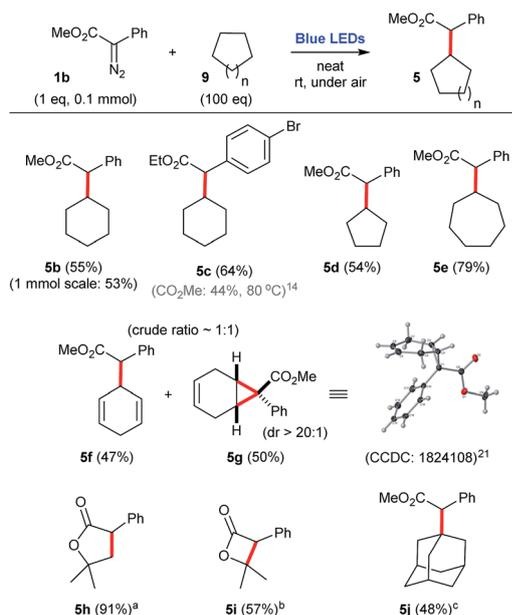
**Scheme 5** C–H insertion reactions employing aryldiazoacetate **1b** and a number of cyclic alkanes and other substrates, under blue light irradiation. <sup>a</sup>Intramolecular process using *tert*-butyl 2-phenyl-2-diazoacetate (0.2 mmol). <sup>b</sup>Intramolecular process using isopropyl 2-phenyl-2-diazoacetate (0.2 mmol). <sup>c</sup>Intermolecular process employing adamantane (5 equiv.).
