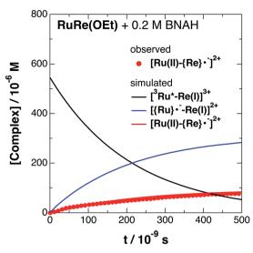
Fig. 4 Time profile of  $[Ru(II)-\{Re\}^{-1}]^{2+}$  (•) in the TRIR measurement of RuRe(OEt) in the presence of 0.2 M BNAH in an argon-saturated CH<sub>3</sub>CN/TEOA (5:1 v/v) solution after 532 nm excitation. The kinetic simulation results for  $[^3Ru^*-Re(II)]^{3+}$ ,  $[\{Ru\}^{-1}-Re(II)]^{2+}$ , and  $[Ru(III)-\{Re\}^{-1}]^{2+}$  are also shown (solid lines).
