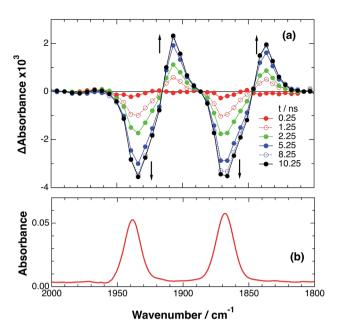
Fig. 6 (a) TRIR spectra (ps-system) recorded after 532 nm excitation of RuRe(FPh) (0.2 mM) in a DMF-TEOA (5 : 1 v/v) solution containing BIH (0.3 M), (b) FT-IR spectrum of RuRe(FPh) in a DMF-TEOA (5 : 1 v/v) solution.
