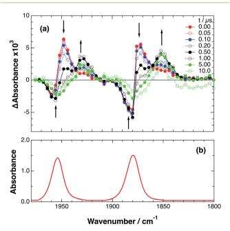
Fig. 1 (a) TRIR spectra (ns-system) recorded after 532 nm excitation of RuRe(OEt) (2 mM) in an argon-saturated CH<sub>3</sub>CN solution. (b) FT-IR spectrum of RuRe(OEt) in CH3CN.
