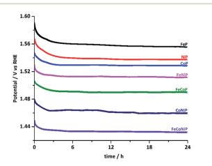
Fig. 4 Chronopotentiometric curves for TMP pre-catalysts recorded at a constant current density of  $10 \text{ mA cm}^{-2}$ .
