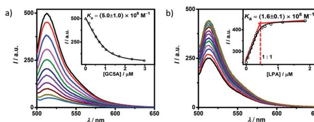
Fig. 1 (a) Direct fluorescence titration of Fl (1.0  $\mu M$ ) with GC5A (up to 3.0  $\mu M$ ),  $\lambda_{em} = 513$  nm. (Inset) the associated titration curve at  $\lambda_{em} = 513$  nm and the fit according to a 1 : 1 binding stoichiometry. (b) Competitive titration of GC5A·Fl (0.4/0.5  $\mu M$ ) with LPA (up to 1.9  $\mu M$ ). (Inset) fit of the titration data to a 1 : 1 competitive binding model. All experiments are in HEPES buffer (10 mM, pH = 7.4) at 25 °C.
