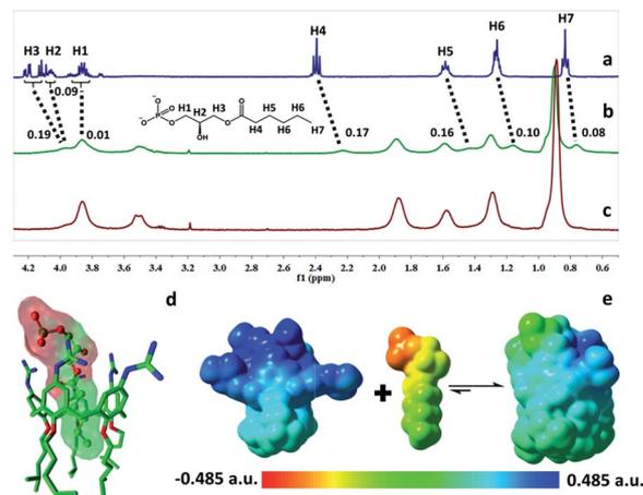
Fig. 2 <sup>1</sup>H NMR spectra of (a) 6:0 LPA (1 mM), (b) 6:0 LPA (1 mM) with addition of GC5A (1 mM), and (c) GC5A (1 mM) in D<sub>2</sub>O at 25 °C. (d) Optimized structure of the GC5A-6:0 LPA complex at the B3LYP-D3(BJ)/6-31G(d)/SMD(water) level of theory. Hydrogen atoms are omitted for clarity. (e) ESP-mapped molecular vdW surface of GC5A, 6:0 LPA and GC5A-6:0 LPA.
