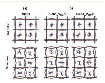
Fig. 15 (a) Defect-free and (b)  $V_{MA}$ -containing defective MAPbI<sub>3</sub> slabs.
