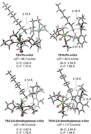
Fig. 13 Optimized structures and the corresponding energy barriers for the transition states of  $\gamma$ -carbon attack (TS3) and Ni-attack (TS10) toward n-OctF for phenyl and 2,6-dimethylphenyl Grignard reagents. Bond distances between key atoms and representative short H–H distances are given.
