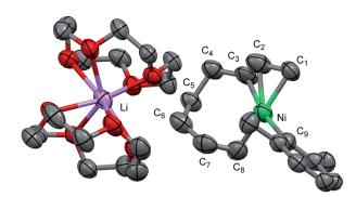
Fig. 2 An ORTEP drawing of one of the four asymmetric units of  $[Ni(C_8H_9)(C_8H_{12}) \cdot Li(12-crown-4)_2]_4(thf)(C_5H_{12})_2$  (8) with thermal ellipsoids at the 50% probability level. All hydrogen atoms and solvent molecules are omitted for clarity.
