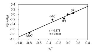
Fig. 9 Hammett plot of the relative reaction rates obtained in the competitive reaction against  $\sigma_{\rm p}^+$ .
