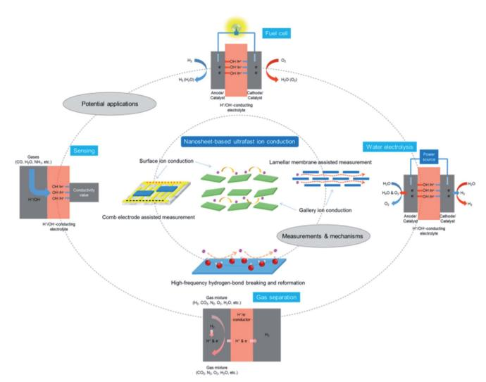
A schematic diagram for the measurements, mechanisms and potential applications of nanosheet-based ultrafast ion conduction.
