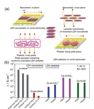
Fig. 6 (a) Schematic drawings for the measurement of different directional hydroxyl ion conductivities for LDH nanosheets and their corresponding bulk precursors. (b) Summary and comparison of the measured conductivities. T: 60 °C and RH: 80%. Reproduced with permission.<sup>31</sup> Copyright 2017, The American Association for the Advancement of Science
