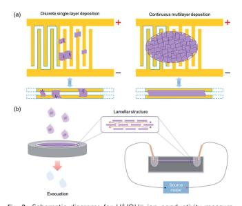
Fig. 2 Schematic diagrams for H<sup>+</sup>/OH<sup>-</sup> ion conductivity measurements in the case of 2D materials. (a) Comb-like microelectrode assisted measurement and (b) lamellar membrane assisted measurement.
