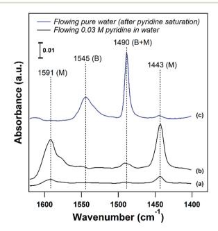
Fig. 3 (a) ATR-FTIR spectra of flowing 0.03 M pyridine in water through the ATR cell devoid of catalyst at 25 °C and (b) through a bed of hydrophilic Si/ZSM-5 at 25 °C. (c) Pyridine adsorbed on H/ZSM-5 (Si/Al =11) after purging with pure water at 75 °C. (B) Brønsted and (M) molecularly adsorbed/bulk.
