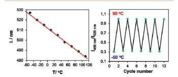
Fig. 7 Left: diagram showing the linear dependence of the emission  $\lambda_{\rm max}$  of BO-1 fluorescence in MOE on T from 223 K (-50 °C) to 383 K (110 °C). Right: diagram showing the reversible cycling of BO-1 emission between -50 °C and 90 °C, plotted with the intensity ratio of  $I_{490~\rm nm}/I_{525~\rm nm}$  vs. T.
