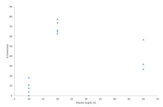
Fig. 3 Reactor length plotted against % conversion to coumalic acid (assessed by  $^1\text{H}$  NMR spectroscopy). Reactions were performed at 70  $^\circ\text{C}$ .
