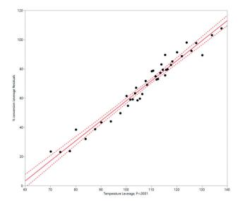
Fig. 10 Modelling the HeRo process, plotting temperature against % conversion estimated by <sup>1</sup>H NMR spectroscopy.
