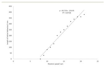
Fig. 7 The effect of rotation speed on the length of the helix at 110
