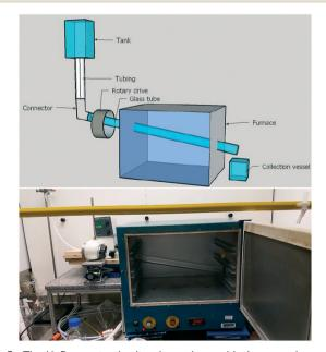
Fig. 5 The HeRo reactor in situ, shown here with the oven door open to demonstrate the placement of the glass work-tube. The dropping funnel and tubing can be seen on the left, leading into the rotary drive which is connected to the work-tube. The material is collected in a flask situated behind the oven door.
