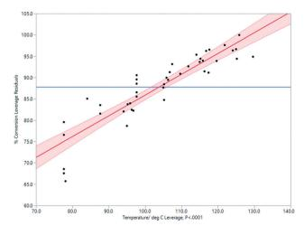
Fig. 4 Impact of temperature on % conversion determined by <sup>1</sup>H NMR spectroscopy in the Vapourtec flow process.
