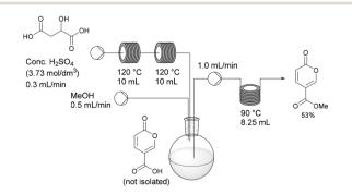
Scheme 9 Small-scale flow procedure for the synthesis of methyl coumalate
