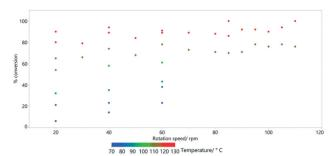
Fig. 8 The effect of rotation speed on % conversion estimated by <sup>1</sup>H NMR spectroscopy for the HeRo process.
