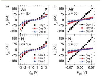
Fig. 2  $I_{\rm DS}/V_{\rm DS}$  characteristics of selected single FGS transistor devices for C/O ratios (a) x=5.4 and (b) x=60 under air (top) and  $N_2$  (bottom) atmosphere at different days. The gate of the device was left unconnected (floating gate).
