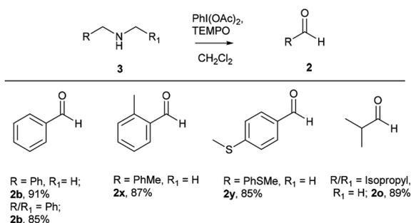
Scheme 3 Oxidation of secondary amines to aldehydes. Reaction conditions unless otherwise specified: amine 1 (1 equiv.),  $\text{PhI}(\text{OAc})_2$  (2 equiv), TEMPO (0.2 equiv), anhydrous  $\text{CH}_2\text{Cl}_2$ , 0 °C to rt, 20 min.
