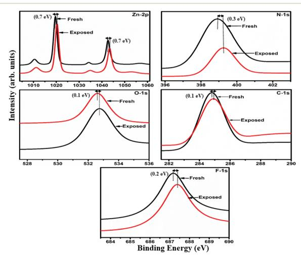
Fig. 14 XPS spectra of the S<sub>2</sub> sensor recorded before and after exposure to 25 ppm of Cl<sub>2</sub>
