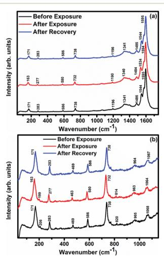
Fig. 11 Raman spectra of the S<sub>1</sub> sensor recorded (a) before exposure (black curve), after exposure (red curve) to 25 ppm of Cl<sub>2</sub> and after full recovery (blue curve); (b) magnified view in the range 30-1300 cm<sup>-1</sup>.
