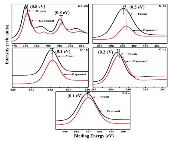
Fig. 13 XPS spectra of the S<sub>1</sub> sensor recorded before and after exposure to 25 ppm of Cl<sub>2</sub>
