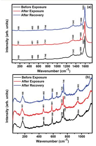
Fig. 12 Raman spectra of the S<sub>2</sub> sensor recorded (a) before exposure (black curve); after exposure (red curve) to 25 ppm of Cl<sub>2</sub> and after full recovery (blue curve) (b) in the range 30-1300 cm<sup>-1</sup> (magnified view).
