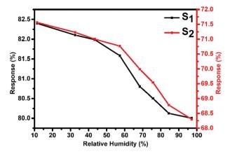
Fig. 10 Variation in the  $Cl_2$  response of  $S_1$  and  $S_2$  sensors with humidity for 2 ppm of Cl<sub>2</sub> at room temperature.
