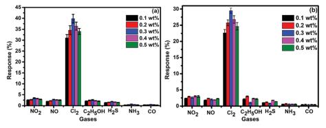
Fig. 8 (a and b) Selectivity histogram of S<sub>1</sub> and S<sub>2</sub> sensors for 500 ppb of NO<sub>2</sub>, NO, Cl<sub>2</sub>, C<sub>2</sub>H<sub>5</sub>OH, H<sub>2</sub>S, NH<sub>3</sub> and CO at room temperature.
