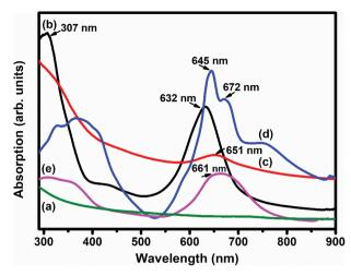
Fig. 5 UV-vis absorption spectra of (a) SWCNTs-COOH; (b) F<sub>16</sub>CoPc; (c)  $S_1$ ; (d)  $F_{16}ZnPc$  and (e) the  $S_2$  hybrid.
