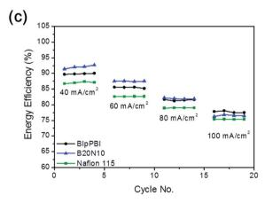
Fig. 6 (a) CE, (b) VE, (c) EE of VRFB single cell performance test.
