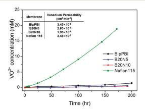
Fig. 3 The vanadium permeability of the membranes.
