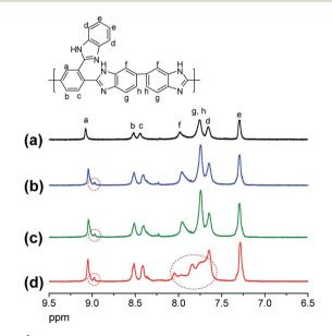
Fig. 5  $\,^{1}$ H-NMR spectra of (a) pristine BIpPBI; (b) B20N5, (c) B20N10, and (d) BIpPBI after  $ex\ situ$  chemical stability test.
