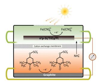
Fig. 2 Schematic of the neutral solar flow battery cell based on a Si photocathode and ferri/ferrocyanide and TEMPO-sulfate redox couples during solar charging. Only the major cation  $(NH_4^+)$  transport through the membrane is shown, though  $K^+$  and  $Na^+$  are the counter ions for the catholyte and anolyte, respectively.
