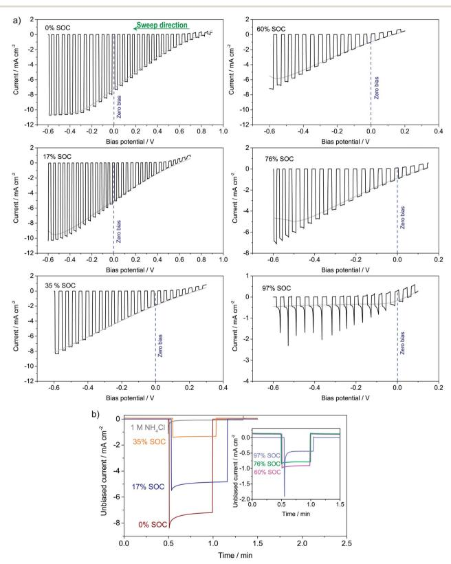
Fig. 6 (a) LSVs on pn $^+$ Si/TiO $_2$  recorded in the solar flow battery cell using the same concentration anolyte and catholyte as in the battery cycling tests. The electrolytes were brought to the indicated SOC in the RFB cell. (b) The unbiased photocurrent density at the same SOCs recorded as the light is turned on (at the time *ca.* 0.5 minute); the inset shows the higher SOCs.
