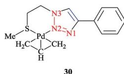
Scheme 19 Structure of the  $[Pd(\eta^3-C_3H_5)(1-(2-(methylthio)ethyl)-4-phenyl-1H-1,2,3-triazole)]^+$  complex (**30**).
