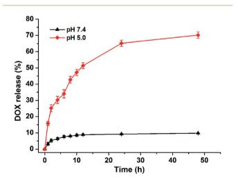
Fig. 5 The cumulative release curve of DOX@ZIF-HA under different pH conditions.
