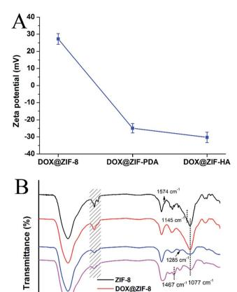
Fig. 4 (A) Surface zeta potential and (B) FTIR spectra of the prepared nanoparticles in different stages.
