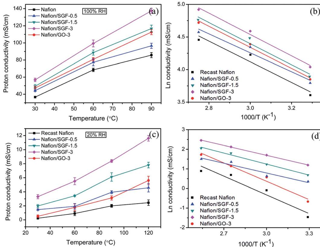
**Fig. 7** Temperature variant proton conductivities of pristine recast Nafion and composite membranes (a) under 100% RH and (c) under 20% RH; corresponding Arrhenius plots of proton conductivities (b) under 100% RH and (d) under 20% RH.
