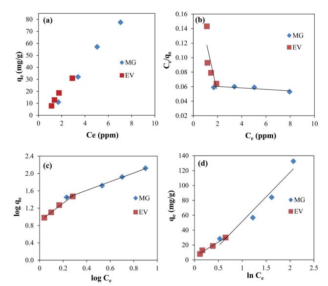
Fig. 4 Plots of (a)  $q_e$  verses  $C_e$ , (b) Langmuir isotherm, (c) Freundlich isotherm, and (d) Temkin isotherm for the adsorption of MG and EV dyes on GO–Au nanocomposite. Reaction conditions; adsorbent = 0.005 g, concentration of dyes solution = 3, 5, 7, and 10  $\mu$ M volume of dyes solution = 50 ml, 100 rpm, 25 °C.
