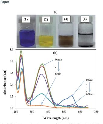
Fig. 9 (a) Photographs of aqueous solutions of (1) ethyl violet, (2) 2-nitroaniline, mixture of ethyl violet and 2-nitroaniline (3) before and (4) after catalytic reduction by using graphene oxide—gold nanocomposite as catalyst. (b) UV-vis absorption spectra showing the simultaneous reduction of ethyl violet dye and 2-nitroaniline in the presence of nanocatalyst.
