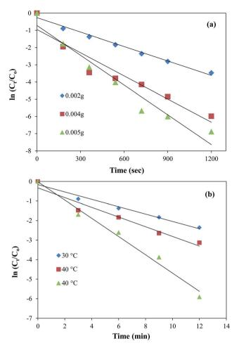
Fig. 8 Dependence of  $k_{\rm app}$  on (a) the amount of catalyst at 30 °C and (b) temperature. Reaction conditions; 0.5 mM aqueous solution of 2-nitroaniline = 50 ml, NaBH<sub>4</sub> = 0.1 g, graphene oxide–gold catalyst = 5 mg, 100 rpm.
