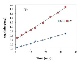
Fig. 5 Plots of (a) pseudo first-order kinetic medal, (b) pseudo second-order kinetic model for malachite green (MG) and ethyl violet (EV) adsorption. Reaction conditions; 7  $\mu$ M solution of each dye = 50 ml, 100 rpm, 30 °C.
