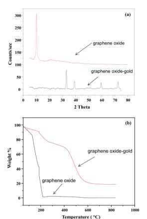
Fig. 2 (a) X-ray diffraction pattern of graphene oxide and graphene oxide-gold nanocomposite (b) thermal gravimetric analysis curves of graphene oxide and graphene oxide-gold nanocomposite.
