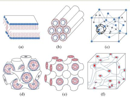
Fig. 1 Schematic representation of the lyotropic liquid crystalline phases commonly found in neutral lipid/water systems. (a) Lamellar phase (b) reverse hexagonal phase (c) reversed micellar cubic of Fd3m (d) reversed bicontinuous cubic (Im3m) (e) reversed bicontinuous cubic (Im3m). (f) reversed bicontinuous cubic (Ia3d).
