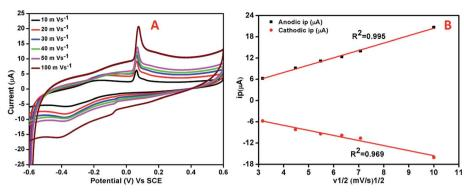
Fig. 8 (A) Cyclic voltammetry curve of AgNPs-rGO-PANI-GCE at different scan rates in PBS [0.1 mM, pH 7.0, 0.5 M KCl], (B) linear variation of anodic and cathodic peak current vs. square root of scan rates.
