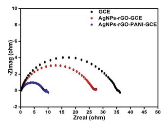
**Fig. 9** (A) Electrochemical impendence spectroscopy in PBS [0.1 mM, pH 7.0, 0.5 M KCI] of AgNPs-rGO, AgNPs-rGO-PANI modified electrode and bare GC electrode.
