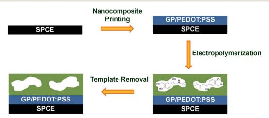
Scheme 1 Schematic representation for the preparation process of electrosynthesized MIP modified nanocomposite based screen-printed carbon electrode (SCPE).
