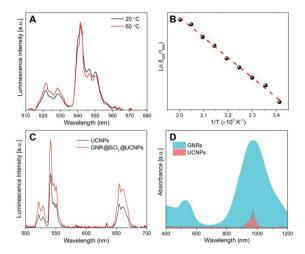
Fig. 3 (A) Normalized upconversion luminescence spectra of UCNPs at two different temperatures. (B) The temperature dependence of the ratio calculated from the luminescence spectra obtained at various temperatures. Dots are experimental results and the red line is the best linear fit. (C) Upconversion luminescence spectra of UCNPs and GNR@SiO2@UCNPs. (D) Normalized absorption spectra of UCNPs and GNRs.
