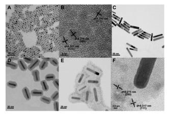
Fig. 1 (A) TEM and (B) HR-TEM images of the synthesized NaGdF<sub>4</sub>: $Er^{3+}$ ,  $Yb^{3+}$ UCNPs. TEM images of the (C) synthesized GNRs, (D) the SiO<sub>2</sub> coated GNRs (GNR@SiO<sub>2</sub>), and (E) the hybrid SiO<sub>2</sub> coated GNRs decorated with NaGdF<sub>4</sub>:Er<sup>3+</sup>, Yb<sup>3+</sup> UCNPs (GNR@SiO<sub>2</sub>@UCNPs), (F) HR-TEM image of the GNR@SiO2@UCNPs interface.
