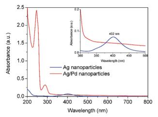
Fig. 5 UV-vis spectra of Ag nanoparticles after Reactor 2 and Ag-Pd bimetallic nanoparticles after Reactor 3 when  $Pd(NO_3)_2$  is used as precursor. All the solutions were diluted 12 times.
