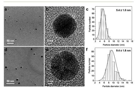
Fig. 2 TEM and HRTEM images and the corresponding particle size distribution histogram of Ag nanoparticles formed in Reactor 1 (a–c) and after growth in Reactor 2 (d–f).
