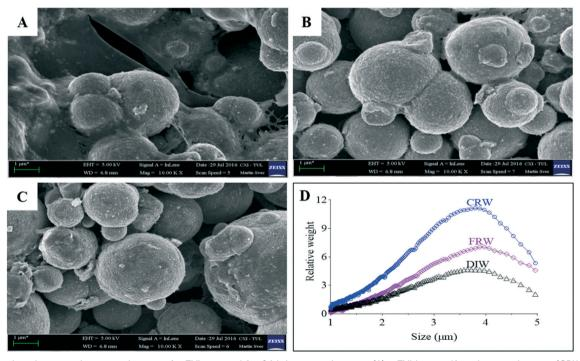
Fig. 2 Scanning electron microscopy images of mZVI exposed for 24 h in reservoir water: (A) mZVI in centrifuged reservoir water (CRW); (B) mZVI in filtered reservoir water (FRW); (C) mZVI in deionised water (DIW) used as a control; scale bar =  $1 \mu m$ ; (D) size distribution of mZVI in CRW, FRW and DIW determined by differential centrifugal sedimentation.
