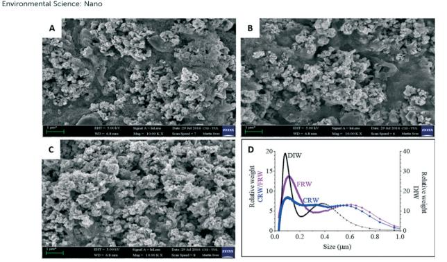
Fig. 1 Scanning electron microscopy images of nZVI exposed for 24 h in reservoir water: (A) nZVI in centrifuged reservoir water (CRW); (B) nZVI in filtered reservoir water (FRW); (C) nZVI in deionised water (DIW) used as a control; scale bar = 1  $\mu$ m; (D) size distribution of nZVI in CRW, FRW and DIW determined by differential centrifugal sedimentation.
