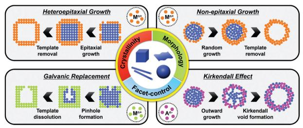
Scheme 1 Representative schematic diagram of synthetic methodologies to hollow nanostructures by using various pre-synthesized templates. The physical and chemical properties of resulting hollow nanostructures are heavily dependent on various factors, such as crystallinity, morphology, dimensionality, and exposed facets, of the engaged templates.
