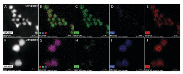
Fig. 10 High-angle annual dark-field (HAADF)-STEM image of CdHg(5)Se (A–E) and CdHg(8)Se (F–J) CQD Cd (green), Hg (blue), and Se (red). Adapted with permission from ref. 63. Copyright 2017 American Chemical Society.
