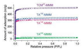
Fig. 19  $N_2$  adsorption/desorption isotherms of  $TA^{105}$ -,  $TA^{150}$ -,  $TA^{200}$ -, and TCM<sup>25</sup>-MMM. The isotherms for the TCM<sup>25</sup>-MMM sample were measured after applying vacuum at room temperature for 4 h. Reprinted (adapted) with permission from ref. 70. Copyright (2018) American Chemical Society.
