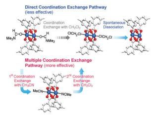
Fig. 8 Schematics illustrating direct and multiple coordination exchange pathways for the activation of the paddle wheel-like (Cu<sup>II</sup>)<sub>2</sub> node of HKUST-1. Hydrogen atoms bound to the carbon atoms in the benzene moieties are omitted for clarity. Reprinted (adapted) with permission from ref. 69. Copyright (2017) American Chemical Society.
