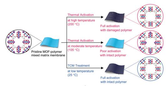
Fig. 17 Schematics illustrating the activation of the paddle wheel-like (Cu<sup>II</sup>)<sub>2</sub> nodes within HKUST-1 by TCM. Hydrogen atoms bound to the carbon atoms in the benzene moieties are omitted for clarity. Reprinted (adapted) with permission from ref. 70. Copyright (2018) American Chemical Society.
