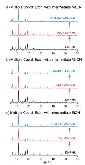
Fig. 12 PXRD patterns of DMF-coordinated HKUST-1 before and after initial solvent treatment with (a) MeCN, (b) MeOH, and (c) EtOH and subsequent solvent treatment with DCM. Reprinted (adapted) with permission from ref. 69. Copyright (2017) American Chemical Society.
