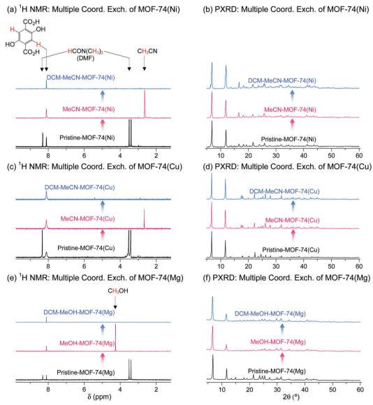
Fig. 15 (a, c and e) <sup>1</sup>H NMR spectra and (b, d and f) PXRD patterns of DMF-coordinated (a and b) MOF-74(Ni), (c and d) MOF-74(Cu), and (e and f) MOF-74(Mg) before and after initial (a-d) MeCN and (e and f) MeOH treatment and subsequent DCM treatment. NMR spectra were measured after the powder samples were completely dissolved in D<sub>2</sub>SO<sub>4</sub>. Reprinted (adapted) with permission from ref. 69. Copyright (2017) American Chemical Society.
