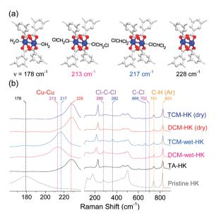
Fig. 2 (a) Schematics of H<sub>2</sub>O-coordinated, DCM-coordinated, TCMcoordinated, and open-state (Cu<sup>II</sup>)<sub>2</sub> centers in HKUST-1 (from left to right). (b) Narrow (left) and wide (right) views of Raman spectra of pristine-HK (gray), TA-HK (black), DCM-wet-HK (pink), TCM-wet-HK (sky blue), dry DCM-HK (red), and dry TCM-HK (blue). Reprinted (adapted) with permission from ref. 70. Copyright (2018) American Chemical Society.
