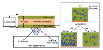
Fig. 3 In situ ion dynamics measurements in IPMC actuators comprising ionic liquid-embedded Nafion™ by ATR-SEIRAS. The enlarged image on the right shows ion detection at the gold/electrode interface during the measurements under a given dc voltage. Figure is adapted from ref. 60 with the permission of American Chemical Society.
