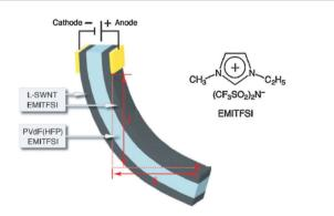
Fig. 4 Schematic bimorph configuration of the actuator strip and chemical structure of the ionic liquid used. Figure is reproduced from ref. 28 with the permission of Wiley-VCH.
