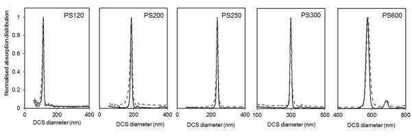
Fig. 3 Normalised light extinction weighted size distributions of the PS NPs as measured by DCS in sedimentation (continuous black line) and flotation (dash grey line) modes. The NPs are assumed perfect spheres of density as in Table 1.
