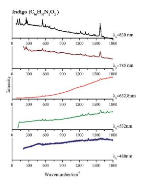
Fig. 14 Raman spectra of indigo.
