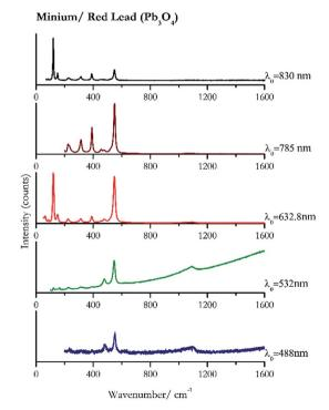
Fig. 1 Raman spectra of minium or red lead.
