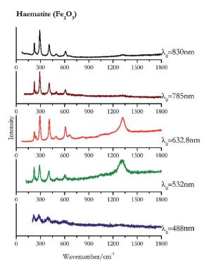
Fig. 2 Raman spectra of haematite.
