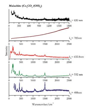
Fig. 24 Raman spectra of malachite
