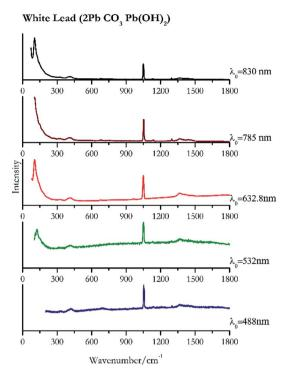
Fig. 22 Raman spectra of white lead.
