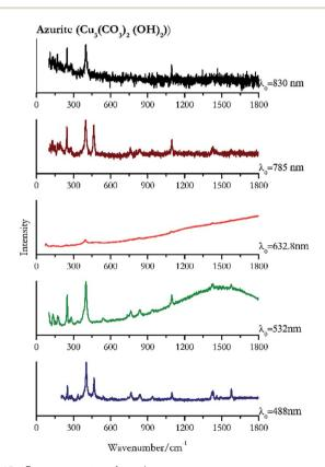
Fig. 15 Raman spectra of azurite.
