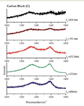
Fig. 25 Raman spectra of carbon black.
