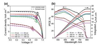
Fig. 3 (a) J-V curves, (b) IPCE and integrated current density of ALD-TiO<sub>2</sub> with thickness 10, 50, 100, 200, 300 and 400 nm, respectively, as a compact HBL for the best PSC.
