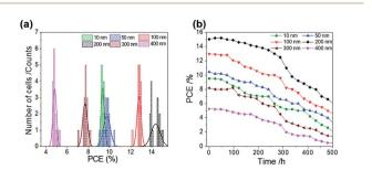
Fig. 7 (a) PCE distribution histogram; (b) PCE evolution of 15 devices stored in ambient air for varied duration/h for ALD-TiO2 of thickness 10, 50, 100, 200, 300 and 400 nm, respectively, as a compact HBL.
