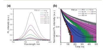
Fig. 5 (a) PL spectra and (b) PL decay profiles of PSK, and PSK deposited on varied compact ALD-TiO $_2$  HBL films. The PL spectra were obtained at excitation wavelength 633 nm; the transient PL decays were obtained using TCSPC with excitation at 635 nm and probe at 770 nm. The fitted results are represented in black lines for all results.
