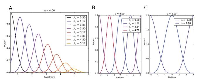
Fig. 2 Examples of the symmetry functions with different parameter sets. (A) Radial symmetry functions, (B) modified angular symmetry functions and (C) the original Behler and Parrinello angular symmetry functions. These figures all depict the use of multiple shifting parameters for each function, while keeping the other parameters constant.
