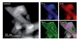
Fig. 3 HAADF-STEM image, Pr-L, O-K, and Ru-L STEM-EDX maps, and reconstructed overlay image of Pr, O, and Ru for Ru/Pr<sub>2</sub>O<sub>3</sub> after H<sub>2</sub> reduction
