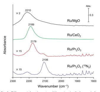
Fig. 6 Difference infrared spectra of  $N_2$  molecules (before and after  $N_2$  adsorption) on supported Ru catalysts. Spectra were collected under 6 kPa of  $N_2$  ( $^{15}N_2$  for Ru/Pr $_2O_3$ ) at 25 °C.
