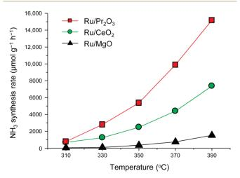
Fig. 2 Rate of NH<sub>3</sub> synthesis over supported Ru catalysts. Reaction conditions: catalyst, 0.2 g; reactant gas,  $H_2/N_2 = 3$  with a flow rate of 60 mL min<sup>-1</sup>; pressure, 0.9 MPa.
