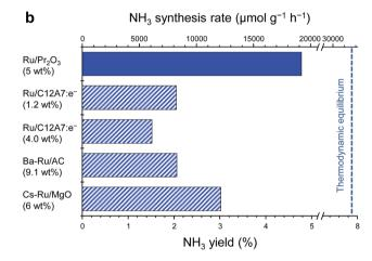
Fig. 1 Catalytic performance of supported Ru catalysts for NH $_3$  synthesis at (a) 0.1 MPa and (b) 1 MPa. Reaction conditions: catalyst, 0.2 g; reactant gas, H $_2$ /N $_2$  = 3 with a flow rate of 60 mL min $^{-1}$ ; reaction temperature, 400 °C. With the exception of Ru/Pr $_2$ O $_3$ , NH $_3$  synthesis rates are reproduced from ref. 10.
