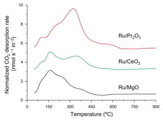
Fig. 5  $CO_2$ -TPD profiles of supported Ru catalysts. Following H<sub>2</sub> reduction at 400 °C,  $CO_2$  adsorption was carried out at 50 °C. These curves show the difference between the curves shown in Fig. S14† to remove the contribution of  $CO_2$  that remained on the surface of the catalysts even after H<sub>2</sub> pre-treatment.
