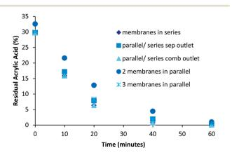
Fig. 3 Influence of reactor design on separation, the determination of residual monomer was performed by <sup>1</sup>H NMR analysis.
