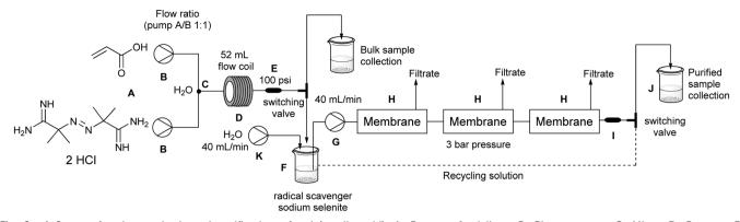
Fig. 8 a) System for the synthesis and purification of poly(acrylic acid); A: Reagent feed lines, B: Piston pumps, C: Mixer, D: Reactor, E: Backpressure regulator, F: Sample collection, G: Peristaltic pump to feed membranes, H: Ultrafiltration membranes, I: Pressure regulator, J: Filtrate of purification, K: HPLC pump used to maintain the sample volume.
