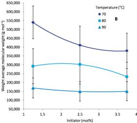
Fig. 5 GPC date: decrease of molecular weight for increase of initiator, the acrylic acid (1) concentration is kept constant at 1.0 mM with A: 5 min residence time and B: 30 min residence time. Other residence times and acrylic acid (1) concentrations show similar trends.
