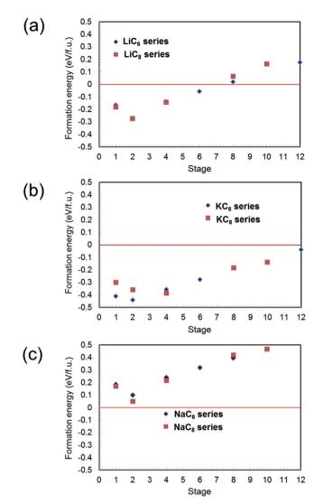
Fig. 1 Calculated formation energies of AM-GICs (AM = Li, Na and K) as a function of stage number for AMC $_6$  and AMC $_8$  series: (a) Li-GIC, (b) K-GIC and (c) Na-GIC.
