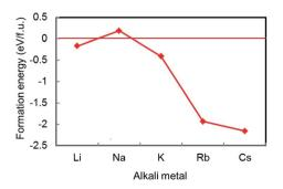
Fig. 2 Calculated formation energies of  $AMC_6$  for AM=Li, Na, K, Rb, and Cs in order of increasing atomic number.
