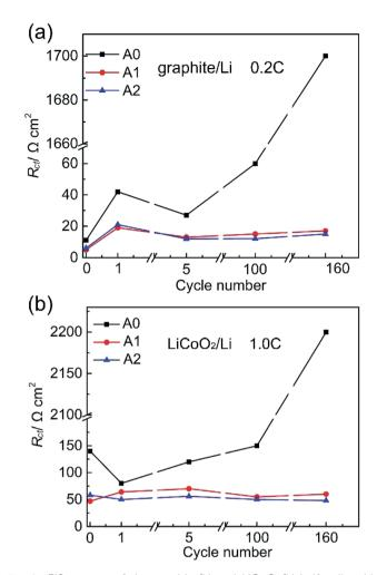
Fig. 2 EIS spectra of the graphite/Li and LiCoO<sub>2</sub>/Li half-cells with electrolytes A0, A1 and A2, after storage for 24 h, 1st, 5th, 100th and 160th cycles at 25 °C. Frequency range of  $10^{-2}$  Hz to  $10^{5}$  Hz with a potential amplitude of 5 mV. (a) The change of the charge-transfer resistances ( $R_{\rm ct}$ ) in the graphite/Li cells. (b) The change of  $R_{\rm ct}$  in the LiCoO<sub>2</sub>/Li cells.
