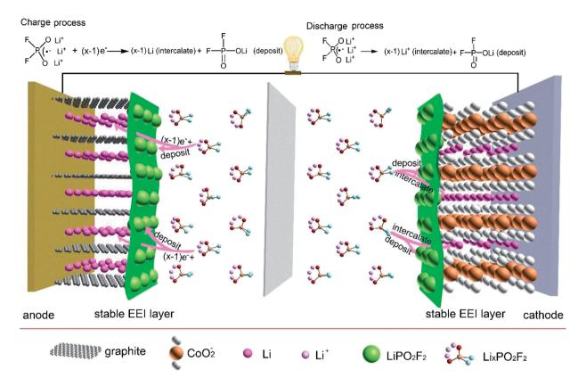
Fig. 6 The schematic of the forming process of SEI on the anode and cathode surfaces in the  $LiCoO_2$ /graphite 18650 full battery with electrolyte containing  $LiPO_2F_2$ , and the reaction on the anode and cathode surfaces during cycle process.
