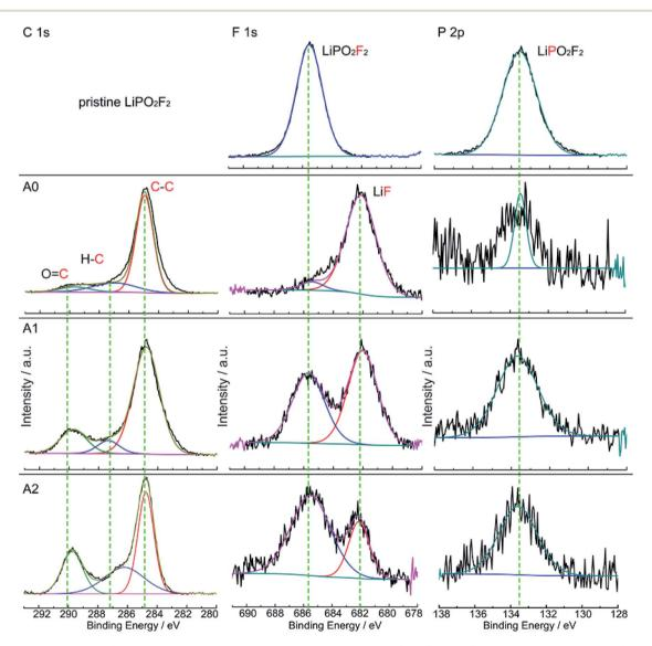
Fig. 5 C 1s, F 1s and P 2p XPS spectra of graphite electrodes from the pristine  $LiPO_2F_2$  (top row), the cell with electrolyte A0, the cell with electrolyte A1, and the cell with electrolyte A2 (bottom row) after 160 cycles at 25 °C.
