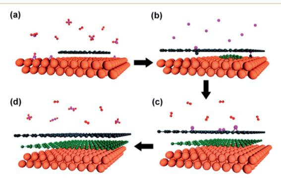
Fig. 64 Schematic of a new bilayer graphene growth protocol. (a) Monolayer graphene is grown *via* standard CVD on Cu surface. (b) Carbon monomer intercalation occurs *via* a penetration mechanism. (c) Hydrogen gas is supplied to etch extra carbon species. (d) With desorption of the hydrocarbons, high-quality bilayer graphene is obtained. This figure has been adapted/reproduced from ref. 200 with permission from American Chemical Society.
