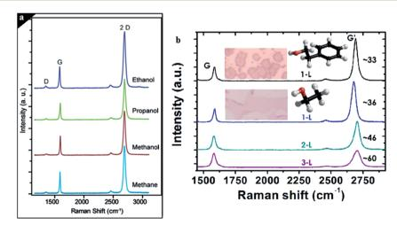
Fig. 4 (a) Comparison of the Raman spectra for graphene film synthesized by methanol, ethanol and 1-propanol. This figure has been adapted/ reproduced from ref. 66 with permission from Elsevier. (b) Raman spectra of single (black and blue lines for 2-phenylethanol and ethanol, respectively), bi (green line) and tri (purple line) layer graphene. This figure has been adapted/reproduced from ref. 61 with permission from Elsevier.
