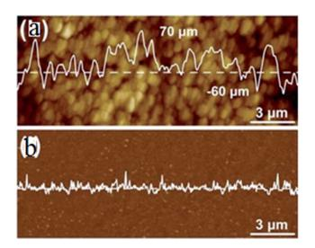
Fig. 57 (a) AFM image of Ni/Mo substrate after annealing at 1000  $^{\circ}$ C, (b) AFM image of graphene transferred onto SiO<sub>2</sub>/Si substrate. Insets are line profiles at the dashed line. This figure has been adapted/reproduced from ref. 179 with permission from Springer.
