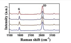
Fig. 3 Raman spectra of the transferred graphene crystal checked randomly at four different areas. Raman spectra show the high crystallinity of a monolayer graphene. This figure has been adapted/reproduced from ref. 27 with permission from Elsevier.
