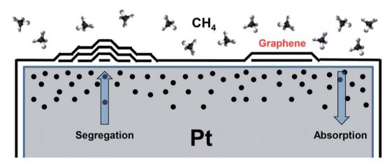
Fig. 60 Schematic of the graphene growth mechanism over Pt surface. Two regimes (balance and segregation) can be defined by the relative strength of carbon deposition, absorption and segregation. This figure has been adapted/reproduced from ref. 194 with permission from American Institute of Physics Publishing.
