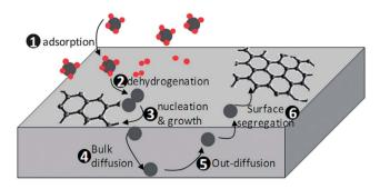
**Fig. 54** Sketch of graphene formation by both direct chemisorption/deposition on Cu and by precipitation/segregation on Ni. This figure has been adapted/reproduced from ref. 180 with permission from The Royal Society of Chemistry.
