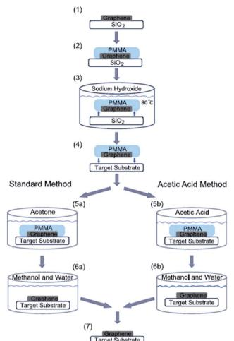
Fig. 13 Schematic of graphene transfer. PMMA was deposited on a graphene layer and cured at  $115\,^{\circ}\mathrm{C}$  for 2 min. The graphene–PMMA stack was then detached from the substrate in a sodium hydroxide bath and subsequently deposited on a target substrate. Finally, the PMMA was dissolved using acetone or acetic acid and then rinsed in a mixture of methanol and water. This figure has been adapted/reproduced from ref. 104 with permission from Elsevier.
