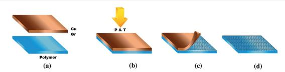
Fig. 26 Schematic of the transfer method and sample after transfer. (a) Graphene/metal and polymer film before transfer. (b) Polymer application step to form the metal/graphene/polymer stack. (c) Peeling of the metal step. (d) Final graphene/polymer stack. This figure has been adapted/reproduced from ref. 125 with permission from Elsevier.
