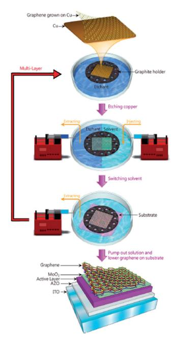
Fig. 15 Schematic of the polymer-free transfer process. This figure has been adapted/reproduced from ref. 105 with permission from American Chemical Society.
