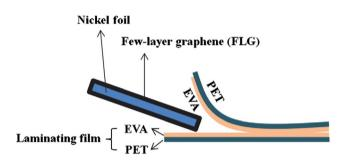
Fig. 30 Schematic of the transfer sample preparation. This figure has been adapted/reproduced from ref. 129 with permission from Elsevier.
