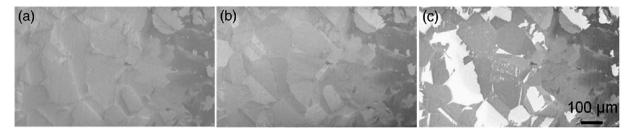
Fig. 40 SEM images showing the contrast for different numbers of layers of graphene on polycrystalline nickel observed at: (a) an elevated temperature during carbon segregation, (b) room temperature without exposure to air, and (c) room temperature after exposure to air. This figure has been adapted/reproduced from ref. 149 with permission from Elsevier.
