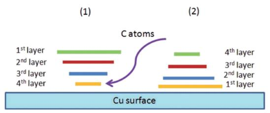
Fig. 65 The proposed model in (1) compared to the model in (2) in terms of schematic side-view of the substrate and multilayer configuration in which the layer growth order, spatial arrangement and relative size are indicated. This figure has been adapted/reproduced from ref. 201 with permission from Wiley-VCH.
