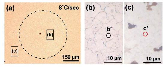
Fig. 56 (a) Low-magnification optical microscope image of as-synthesized graphene on Ni/SiO $_2$ /Si substrate using 2 sccm CH $_4$ , 30 s growth duration and a fast cooling process. (b) & (c) High-magnification images of the regions corresponding to the region in (a). Dashed circle in (a) presents a boundary where graphene is synthesized. This figure has been adapted/reproduced from ref. 179 with permission from Springer.
