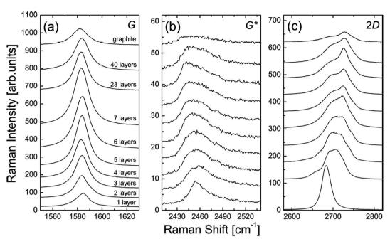
Fig. 33 Evolution of the: (a) G band, (b) G\* band, and (c) 2D band in the Raman spectra as functions of the number of graphene layers. This figure has been adapted/reproduced from ref. 133 with permission from Springer.
