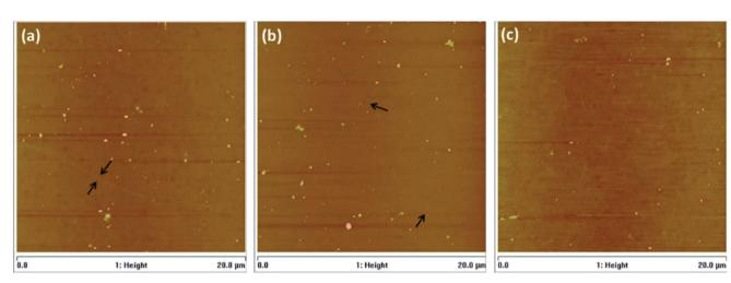
Fig. 16 AFM images of graphene films baked during: (a) 5 min at 80 °C, (b) 5 min at 80 °C + 20 min at 130 °C and (c) 5 min at 80 °C + 40 min at 130 °C. This figure has been adapted/reproduced from ref. 106 with permission from Elsevier.
