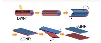
Fig. 6 Method of synthesizing single-layer graphene nanoribbons (sGNR) from double-walled carbon nanotubes (DWCNTs). This figure has been adapted/reproduced from ref. 71 with permission from Nature Publishing Group.
