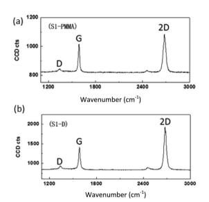
Fig. 23 Raman spectra (532 nm laser excitation wavelength) for graphene transferred onto the  $SiO_2$ -on-Si substrate. (a) Raman spectra obtained from a sample prepared by the standard PMMA-based method. (b) Raman spectra obtained from a sample obtained by the direct transfer method. This figure has been adapted/reproduced from ref. 123 with permission from World Scientific.
