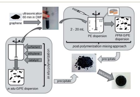
Fig. 4 Preparation of PE/graphene composites by *in situ* polymerization, post polymerization mixing and precipitation methods (reproduced with permission from ref. 58 *copyright* 2014 American Chemical Society).
