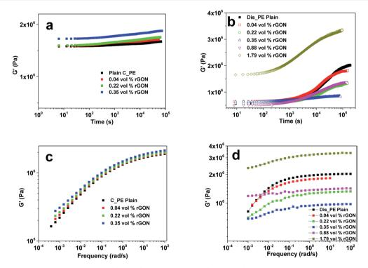
Fig. 7 Storage modulus vs. frequency graphs of (a) C\_PE/rGON composites. (b) Dis\_PE/rGON composites and frequency sweep graphs of (c) C\_PE/rGON composites. (d) Dis\_PE composites (reproduced with permission from ref. 79 copyright 2015 American Chemical Society).
