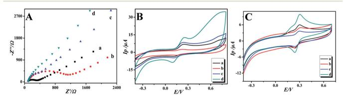
Fig. 3 Electrochemical impedance spectroscopy recorded in 0.2 mM  $K_3$ [Fe(CN)<sub>6</sub>] solution (A). Cyclic voltammograms showing the response of different modified electrodes to 1  $\mu$ M DA (B); 1  $\mu$ M DA and 40  $\mu$ M AA (C) in 0.1 M PBS. (a) GCE, (b) GO/GCE, (c) GO-IL/GCE, and (d) GO-IL-AuNPs/GCE.
