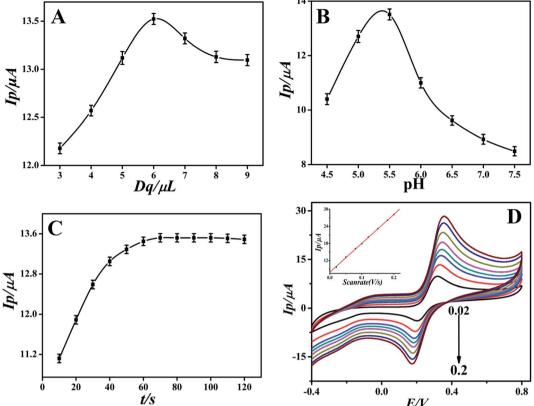
Fig. 4 (A) Effect of the volume of GO-IL-AuNPs. (B) Effect of pH value. (C) Effect of accumulation time. (D) CVs of GO-IL-AuNPs/GCE in 0.1 M PBS (pH 5.5) with 10  $\mu$ M DA at different scan rates (0.02, 0.05, 0.08, 0.1, 0.12, 0.15, 0.18, and 0.2 V s<sup>-1</sup>). Inset: the linear relationship between peak current and scan rate.
