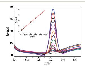
Fig. 5 Differential pulse voltammograms of different concentrations of DA at GO-IL-AuNPs/GCE (pH = 5.5). Inset: linear calibration curve in the range 7 nM to 5  $\mu$ M DA.
