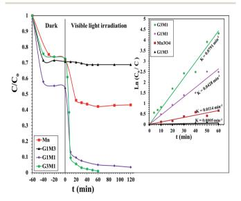
Fig. 6 Photocatalytic degradation of the MB dye by Mn<sub>3</sub>O<sub>4</sub>, G3M1, G1M1 and G1M3 photocatalysts under visible light irradiation: reaction conditions: (lamp power = 88 W, filter  $\lambda$  = 420 nm, catalyst weight 100 mg, dye conc. 20 ppm). Insets are the kinetic fits for MB degradation *via* the as-synthesized photocatalysts.
