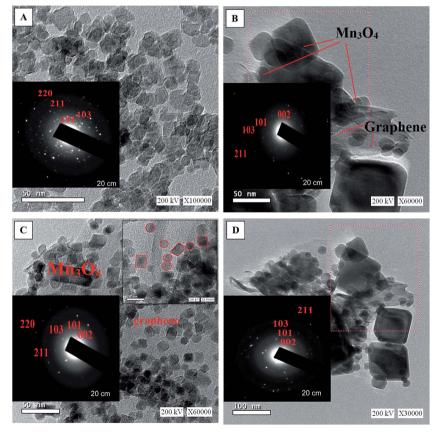
Fig. 2 TEM images of (A)  $Mn_3O_4$  (B) G1M1 (C) G3M1 and (D) G1M3 together with the corresponding magnified HRTEM images and SAED patterns, as insets.
