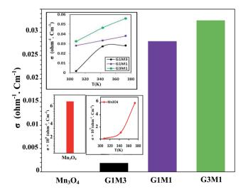
Fig. 12 Conductivity results of Mn<sub>3</sub>O<sub>4</sub>, G3M1, G1M1 and G1M3 samples measured at room temperature and at 373 K. Inset is the  $\sigma$  vs. T for exploring the effect of increasing temperature on the conductivity.
