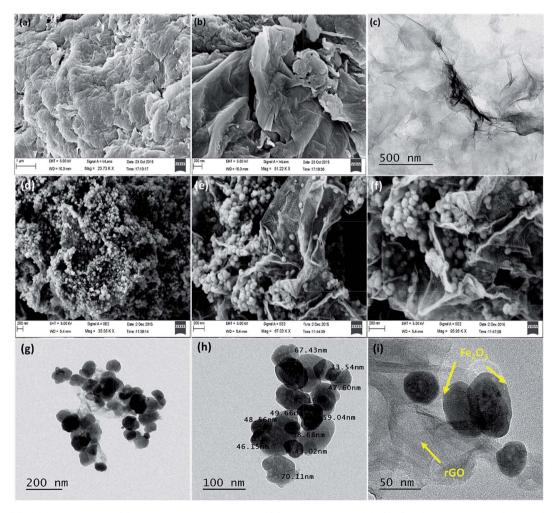
Fig. 2 (a) and (b) FESEM images of rGO at different magnifications, (c) TEM image of rGO, (d-f) FESEM images of rGO-Fe<sub>2</sub>O<sub>3</sub> composite at different magnifications, and (g-i) TEM image of rGO-Fe<sub>2</sub>O<sub>3</sub> composite at different magnifications.
