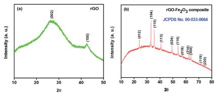
PXRD spectra of (a) rGO and (b) rGO-Fe<sub>2</sub>O<sub>3</sub> composite.
