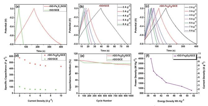
Fig. 5 (a) Comparison of GCD profiles of rGO/GCE and rGO $-Fe_2O_3$ /GCE at a current density of 2 A  $g^{-1}$ , (b) and (c) GCD profiles of rGO and rGO $-Fe_2O_3$ /GCE at different current densities, (d) specific capacitance as a function of current density for rGO/GCE and rGO $-Fe_2O_3$ /GCE, (e) capacity retention of rGO/GCE and rGO $-Fe_2O_3$ /GCE for 1000 cycles in 1 M Na<sub>2</sub>SO<sub>4</sub>, and (f) Ragone plot for rGO $-Fe_2O_3$ /GCE.
