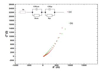
Fig. 6 Nyquist plots for (a) rGO-Fe<sub>2</sub>O<sub>3</sub>/GCE and (b) rGO/GCE vs. Ag/ AgCl over the frequency range of 1 Hz to 60 kHz in 1 M Na<sub>2</sub>SO<sub>4</sub>. Here Z'= real impedance and Z'' = imaginary impedance, inset shows the equivalent circuit.
