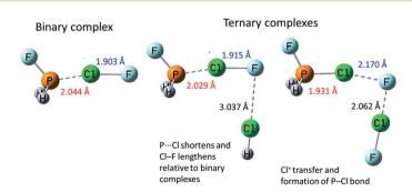
Fig. 4 Computational models of complexes  $H_2FP\cdots ClF$ ,  $H_2FP\cdots ClF\cdots ClH$  and  $H_2FP\cdots ClF\cdots ClF$ , illustrating co-operativity in halogen bonding interactions. Adapted from DOI: 10.1039/c7fd00048k with permission from The Royal Society of Chemistry.
